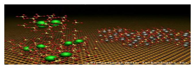
This figure shows a lot of hardness crystals formed on RO membrane in which no RO antiscalant is used
